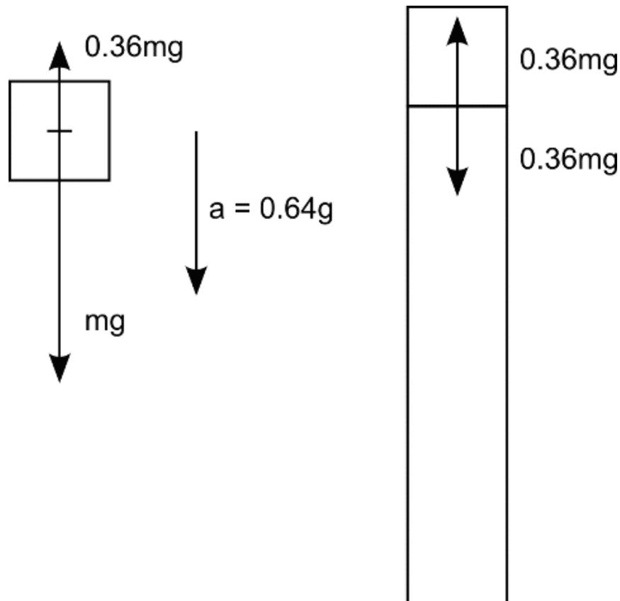
Figure 3: Consider the upper section of the building to be a block of weight  $mg$ . Since the acceleration of the block is measured to be downward at  $0.64g$ , the net force acting on it must be  $0.64mg$ . The gravitational force is  $mg$ , so the upward normal force must be  $0.36mg$ . The upper and lower sections of the building exert equal but opposite forces on each other, so the load on the lower section of the building is 36% of the weight of the upper block.
